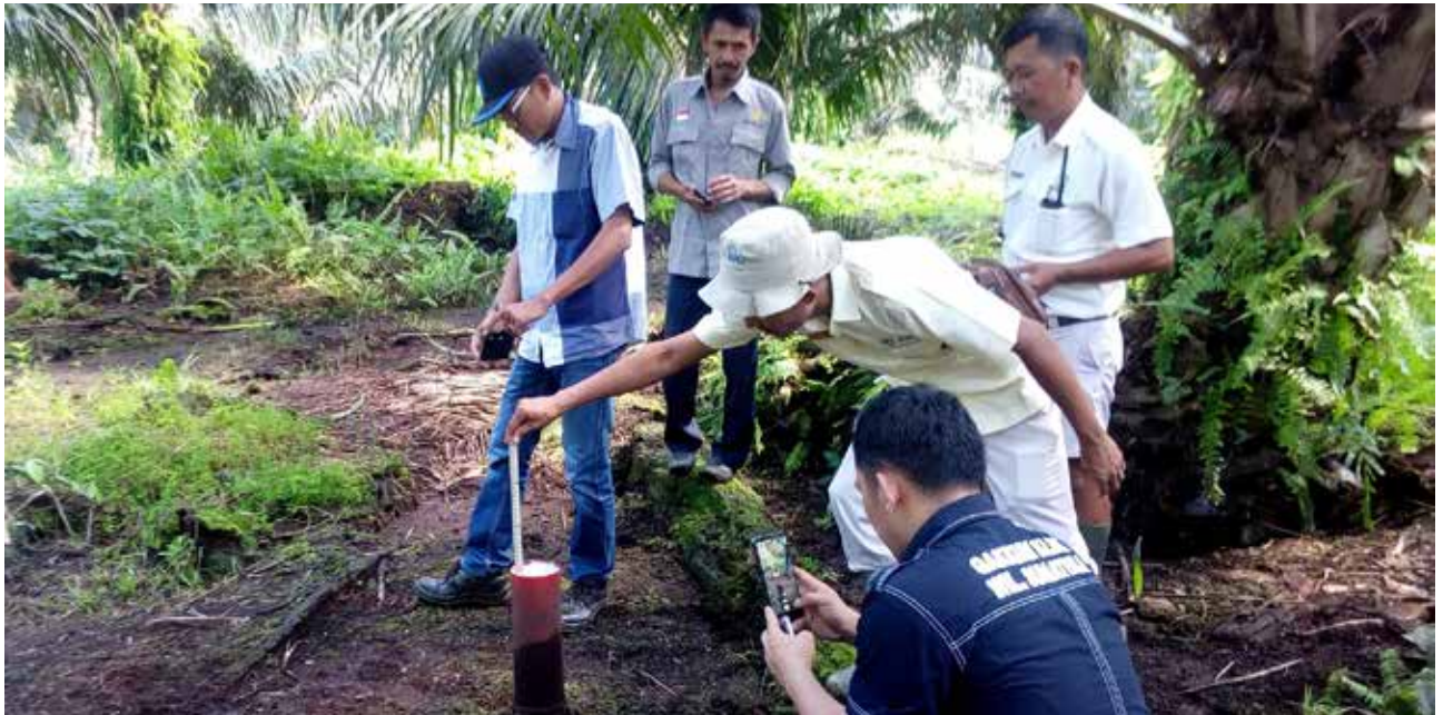
Measuring the rate of subsidence and water table height in a peatland area.
