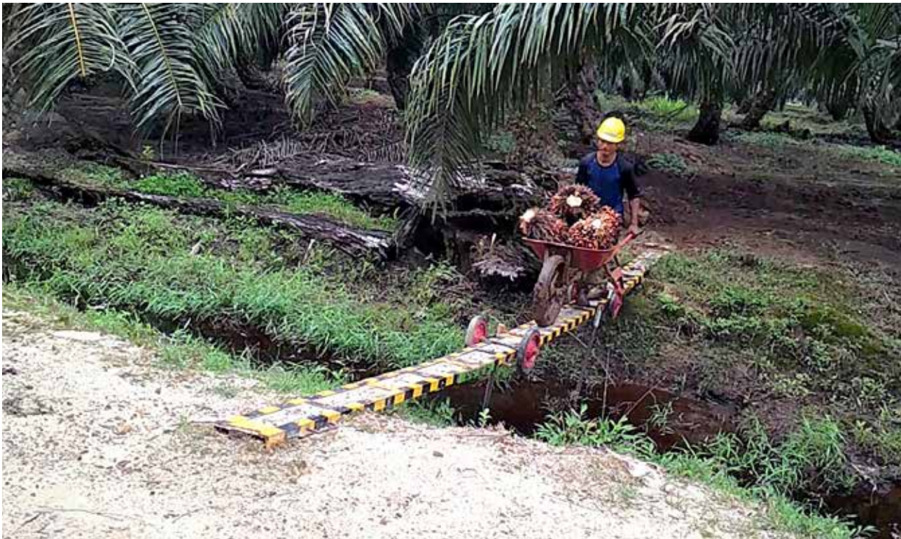
Portable footbridges for harvesting and compost application named 'Titi PUSPA', an initiative of Quality Improvement Project from ANJAS.
